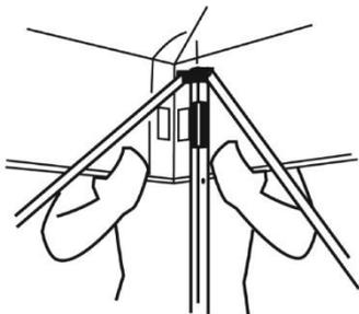
Falt the frame untill the middle and take of the clam of the peak pole, Unattach the velcro of the corners
