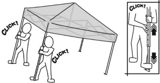
Lift each leg and slide lower leg extension out until the latching button snaps into the first adjustment
