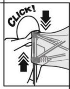
Depress push button on upper legs, pull down safety lock, you will feel that the pressure of the roof is gone.
