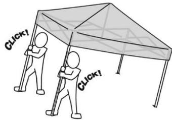
Depress push button on lower leg to collapse teh other legs all down
