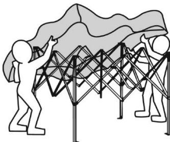
Take of the roof of the frame and fold this properly
