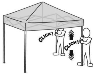
Depress push button on lower leg and collapse 2 legs all down.
