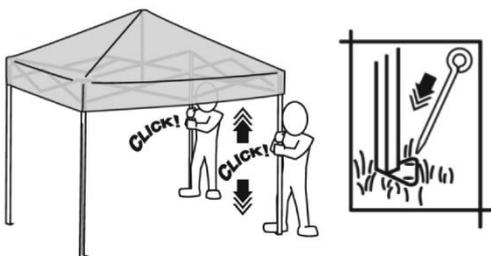
Attach the roof on the frame (inside) with the clams. You can adjust the height like the height you want.
